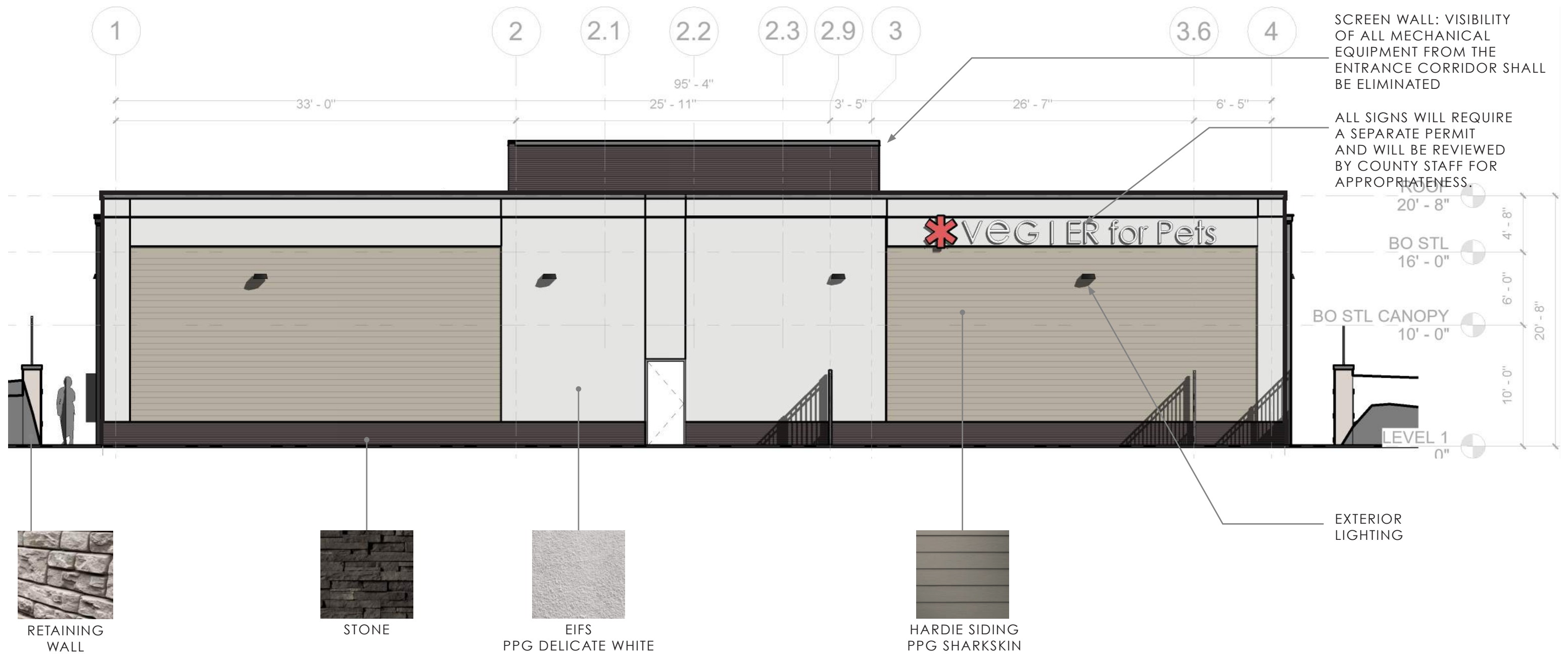
SOUTH ELEVATION - ALONG HYDRAULIC ROAD
